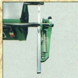
▶ Quick action swing away rip fence for accommodating larger panels.
