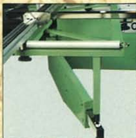
▶ Efficient 100mm (4") diameter dust extraction outlet.
