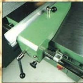
▶ Heavy duty rip fence with quick action locks and micro adjustment positioning complete with magnifier for accurate scale reading.
